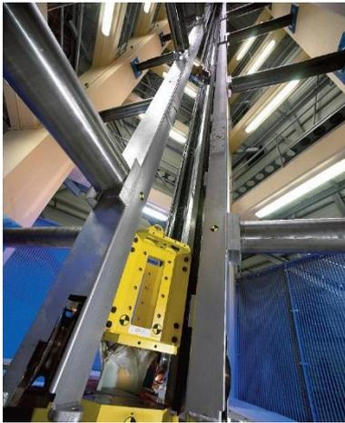
Crash tower to test the structures' resistance
