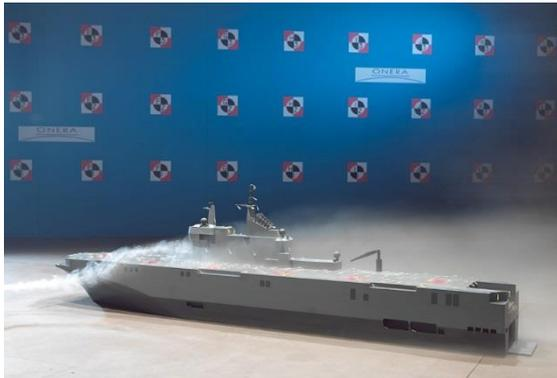
The L2 large wind tunnel with its atmospheric boundary layer
