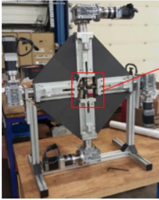
In-plane biaxial tension (large load, small strain)
