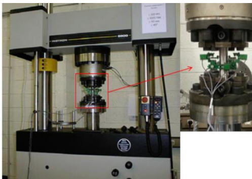
Tension-Torque- internal pressure 100kN/100 Nm / 100 bar
